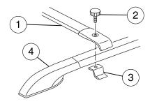
2. Align the clamps (3) under the side rails (4) and install the thumbwheels (2) through the cross bar (1) and side rails (4) into the clamps (3). Repeat steps 1 and 2 to install the other cross-bar.
